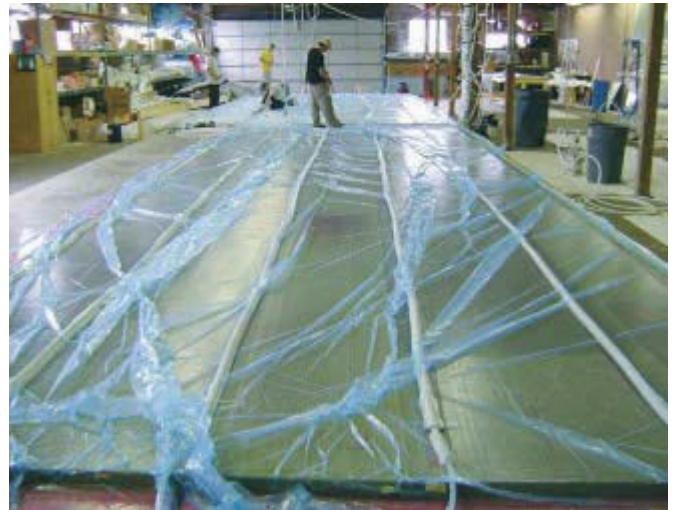
Above left —A curved structural bulkhead, positioned on its side, is being infused on a one-off plywood mold. The red area is a doorway. Above right —The crew can infuse one 18' x 39' (5.5m x 12m) flat Divinycell-cored panel per day. A Gurit/SP epoxy resin permits compliance with less-stringent fire codes (styrenated resins' flashpoints are too low). Left —The floor of the lamination room is actually a large (80'/24.4m) heated table for initiating the cure of infused parts. Many parts that Gardiner currently makes are of carbon pre-preg; the material is stored in a refrigerated outbuilding until needed on the shop floor.
